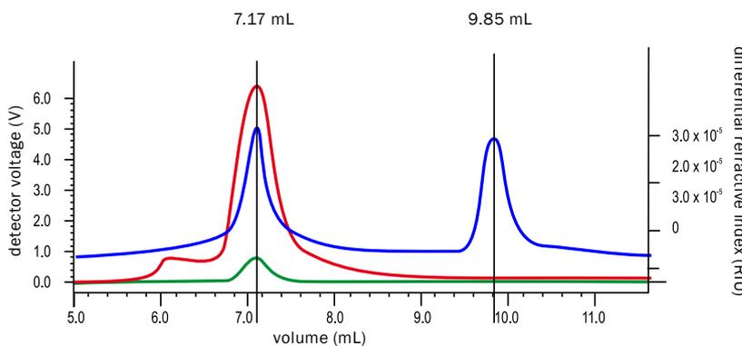
**SAMPLE 1:** Dimeric Photosystem II (PSII) membrane protein concentrated 273 times. Note the free detergent micelles eluting at 9.85 ml.
