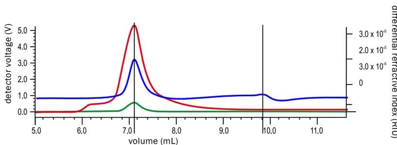
**SAMPLE 2:** SAMPLE 1 after elution from the Proteus Detergent Anion Exchange Mini Spin Column with 75 mM MgSO<sub>4</sub> in detergent-depleted buffer. Note the effectiveness of the Proteus spin columns to eliminate free detergent micelles.
